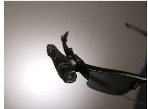
Body-worn cameras can be worn by officers using a variety of mounting options
